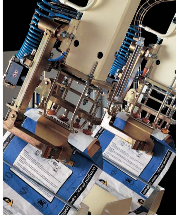
Close-up of tilting-arm bag applicator.
