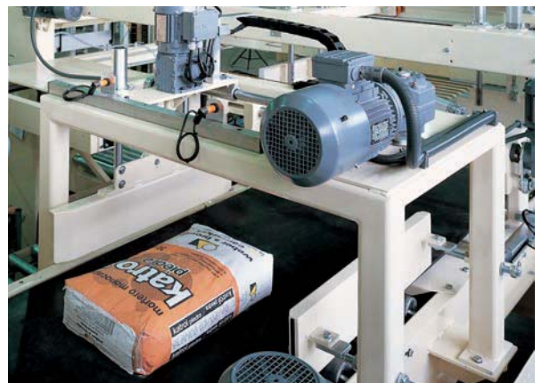
Electric bag shifter, driven by a connecting rod – crank system.
